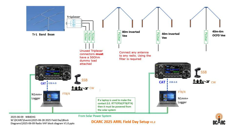
These are our HF radios and antennas. We operated as 2A where the 2 is the number of transmitters on the air at any one time. Any unused antenna can be routed to the building which would allow us to put that station on the air.
