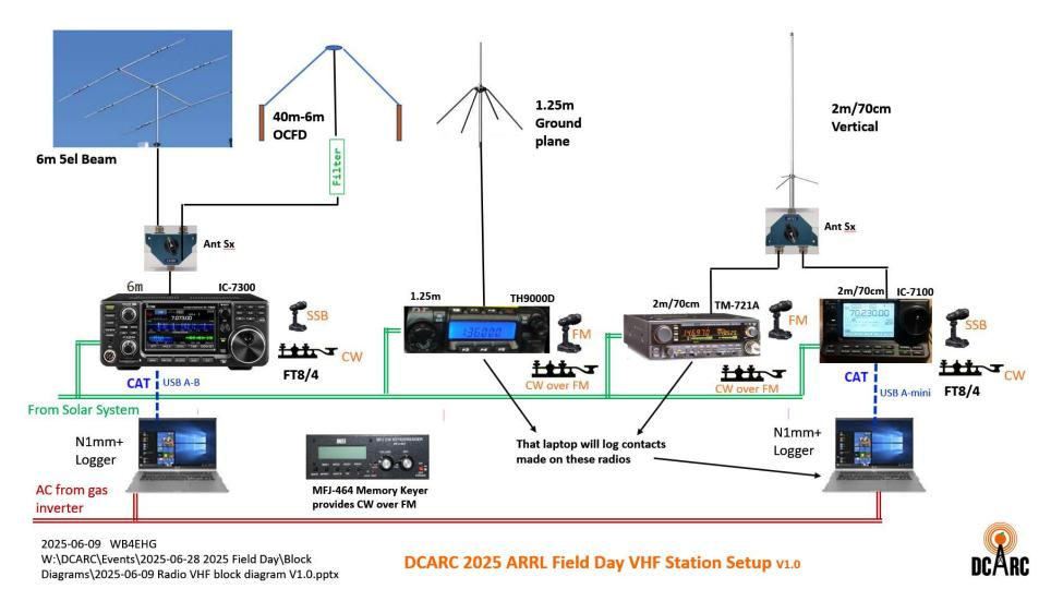
This is the VHF/UHF station that was in the building. I went a bit overboard setting up four radios. This setup is more useful for the events that use band-mode multipliers. The 6m station (IC-7300) made a lot of contacts. The TH9000D (1.25m) and TM-721 (2m/70cm) were examples of a VHF/UHF home station. We made FM phone and CW over FM contacts from these stations.
